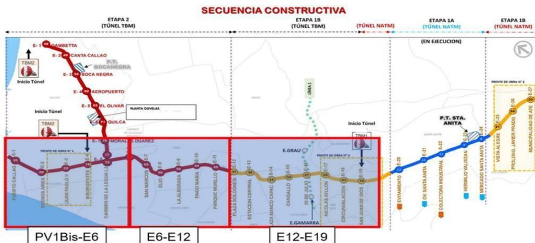
Figure 1. Layout of Line 2 and part of Line 4 of the Lima Metro with associated stations and the distribution of the sections according to the type of excavation; marked red: TBM stretch of Line 2.
