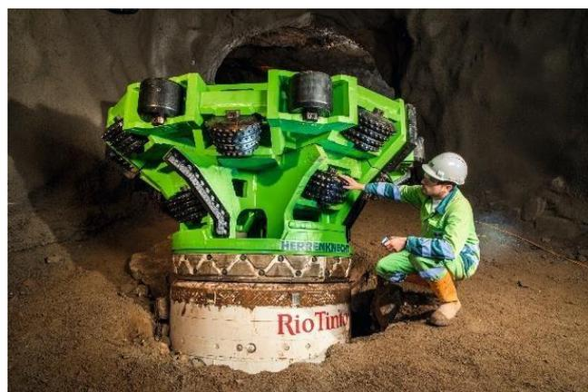
Figure 11. Reamer head before starting the reaming process
