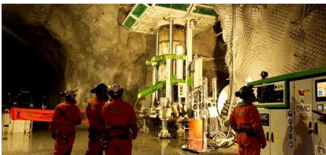
Figure 13. Operation of BBR1500 in El Teniente mine in Chile (Picture: DMC Chile)
