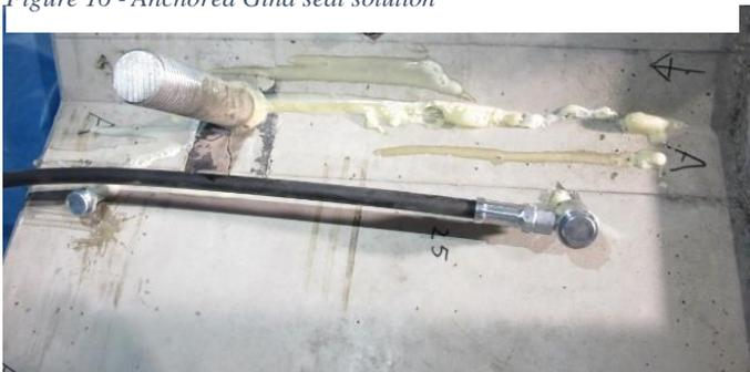
Figure 17 - Pre-casted injection tubes in anchored Gina concept
