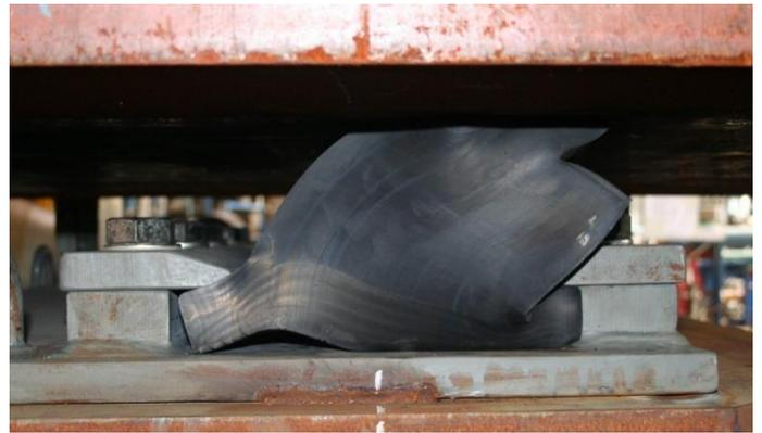
Figure 9 - 150 mm transverse shear movement
