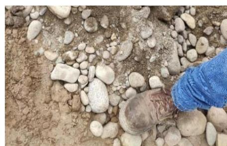
Figure 3. Gravas of Lima, with significant portions of cobbles and boulders.
