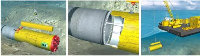
Figure 2. Recovery of a tunnelling machine from the seabed.
