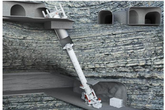
Figure 12. Top-down lining process and reaming
