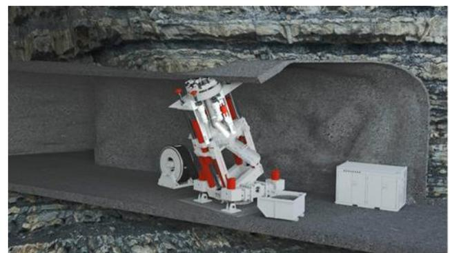
Figure 10. Illustration of the working principle of the BBR (pilot hole drilling)
