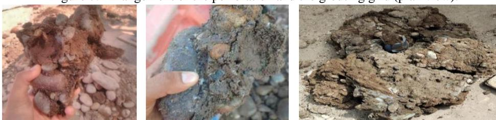
Figure 8. Results of the test grouting, bonded subsoil samples.
