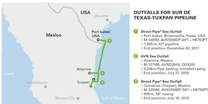
Figure 6. Overview on Sur de Texas-Tuxpan gas pipeline landfalls.
