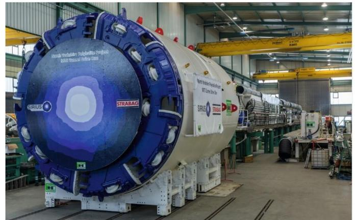
Figure 2. Factory acceptance of the 5.94m-diameter Single Shield TBM in Germany.
