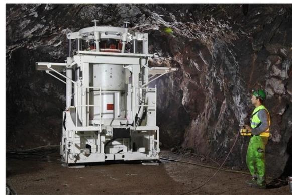
Figure 5. During excavation the system is operated by remote control, without any personnel in the danger zone
