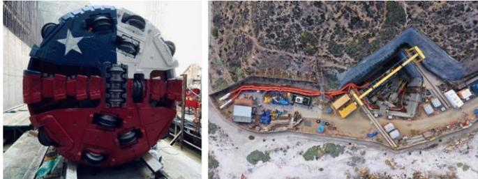
Figure 5. Upskinned AVN1800 with hard rock cutting wheel and jobsite installation on the coast.
