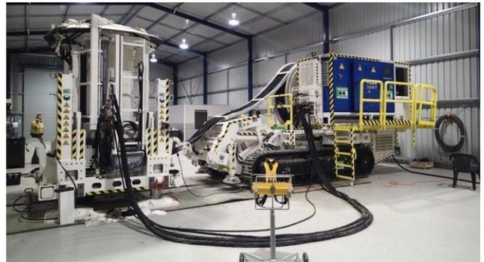
Figure 2. Herrenknecht Boxhole Boring Machine (BBM) in the customer factory
