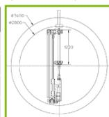
As shown in Table 4, the minimum tunnel diameter for a drilling campaign driven from inside a tunnel is about 2.8 m. For a reasonable drilling campaign of 15-20 m above the tunnel roof, an individual feed length of 4 ft (1220 mm) is recommended. For a total drill length of 20 m, more than 16 drill rods need to be used which requires 15 extension intervals. Since several drillings are required along the tunnel cross
